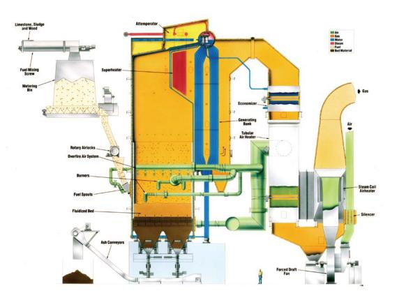
$B\&W\spaces$  open-bottom BFB design allows the removal of non-combustible material from the furnace while the boiler is operating.
