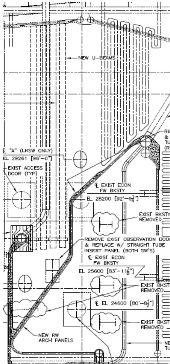
**Figure 5.** External U-Beams and Particle Transfer Hopper After Retrofit
