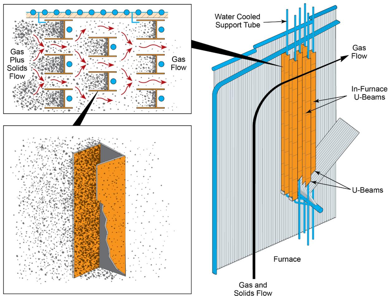
**Figure 3.** Views Showing Flue Gas and Solids Flow Through U-Beams
