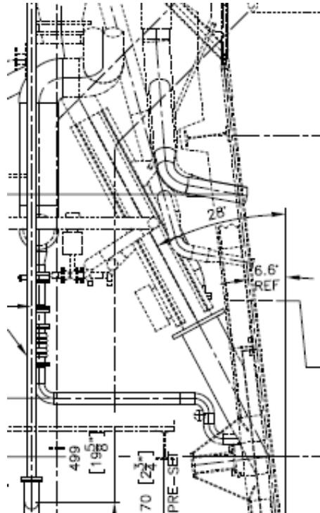
**Figure 7.** Coal Chutes and Motive Air Piping After Retrofit
