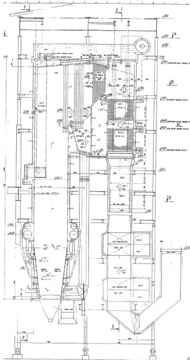
**Figure 1.** Sectional Side View of Existing IRPC CFB Boiler
