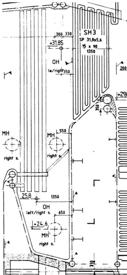
**Figure 4.** External U-Beams and Particle Storage Hopper Before Retrofit
