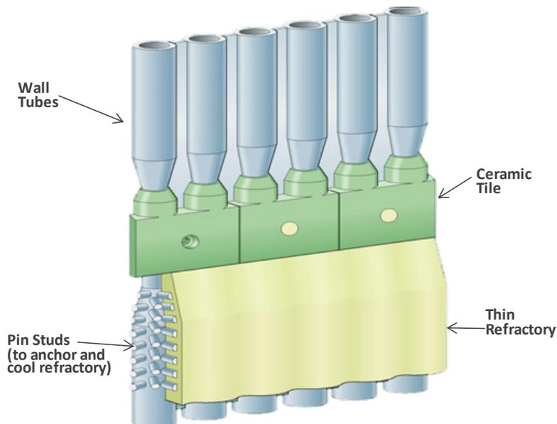
**Figure 8.** Reduced Diameter Zone at the Refractory Transition in Lower Furnace
