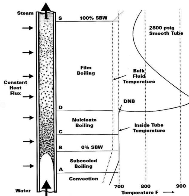
Figure 12. Characteristics of Departure from Nucleate Boiling
