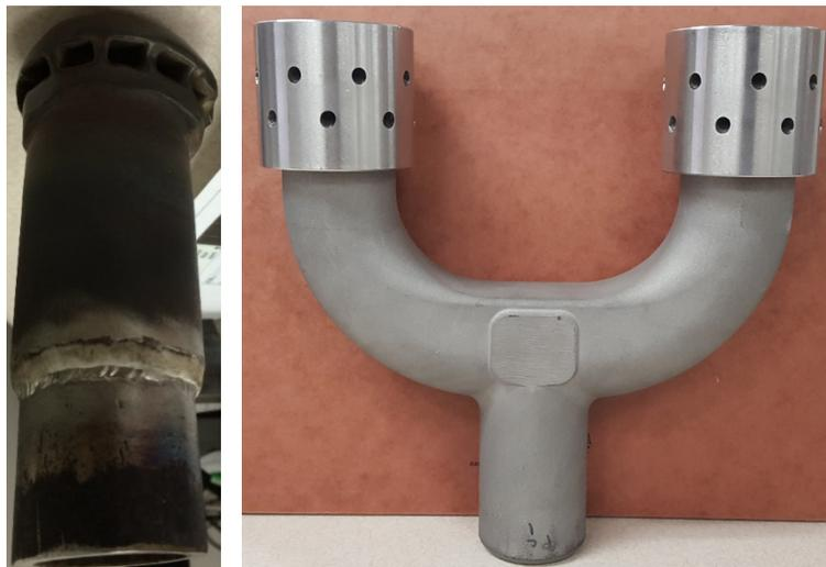
**Figure 13.** Original Bubble Cap Design (Left) and New Bubble Cap and Bifurcate Design (Right)
