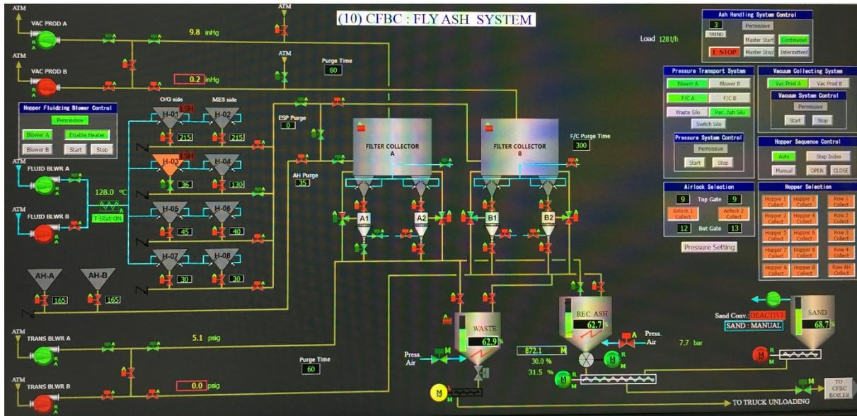
**Figure 6.** Secondary Solids Capture and Recycle System Schematic
