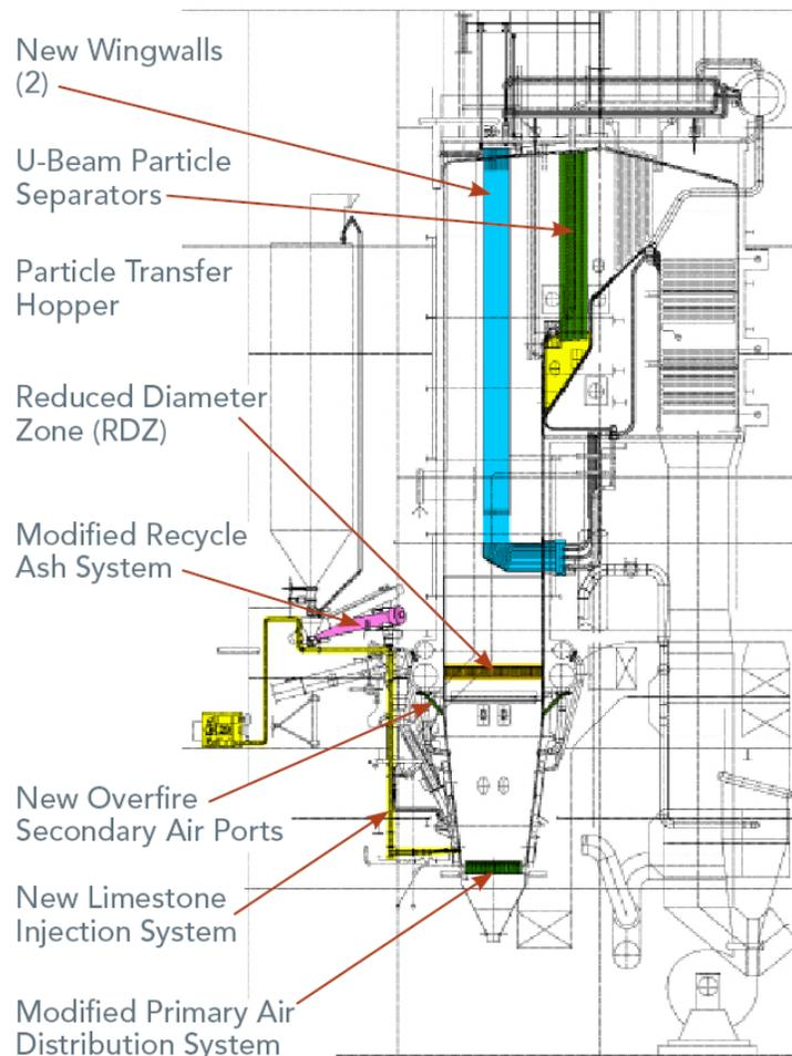
**Figure 2.** Primary Boiler Modifications
