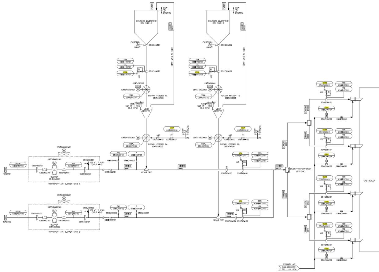
**Figure 14.** Pneumatic Limestone Feed System Schematic
