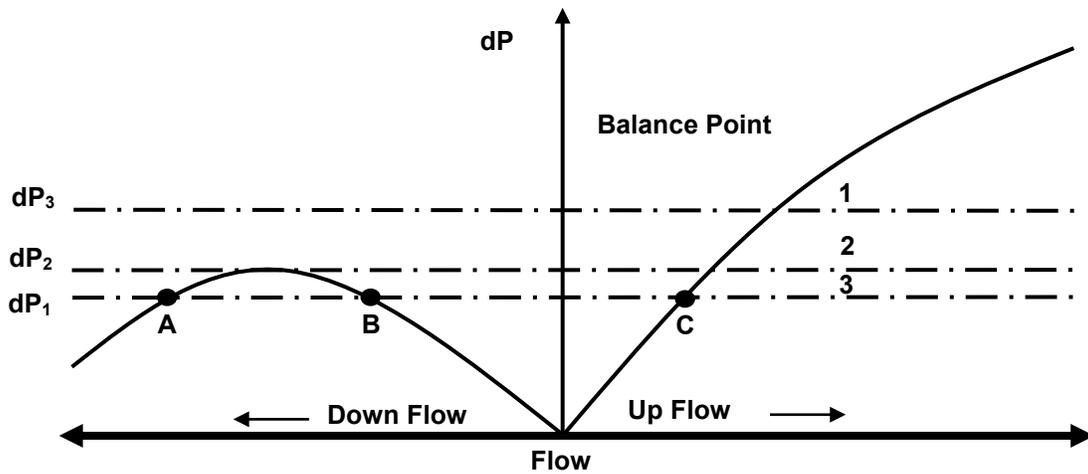
Figure 11. Pressure Drop Characteristics of a Boiler Tube
