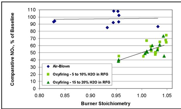
Fig. 3 NO<sub>x</sub> emissions for lignite.
