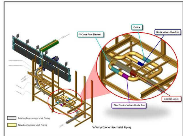
Fig. 3 Expanded view of V-Temp system.
