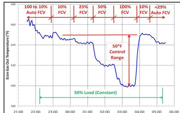
Fig. 12 CV-1 position vs EGT.
