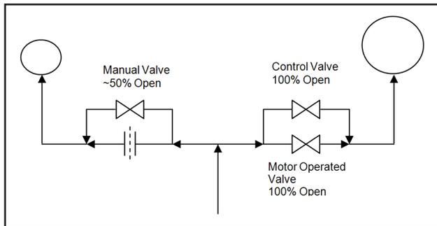
**Fig. 6** Valve positions – all loads above the SCR MAIT (including full load).
