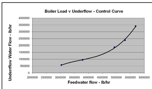
Fig. 10 Control curve – boiler load vs underflow rate.
