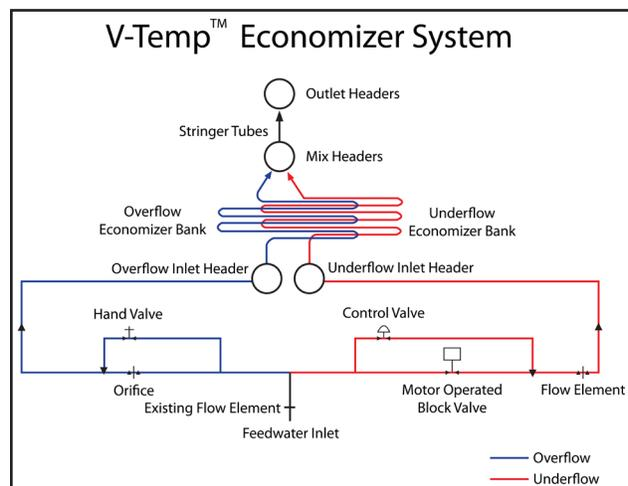
Fig. 1 V-Temp economizer system schematic.
