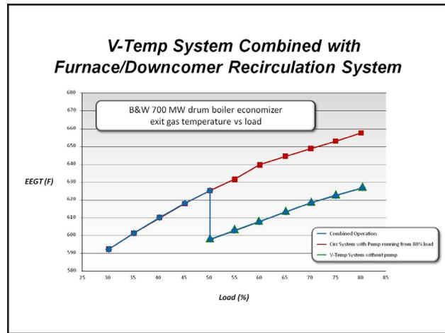
Fig. 14 Furnace/downcomer recirculation system performance curve with V-Temp system.
