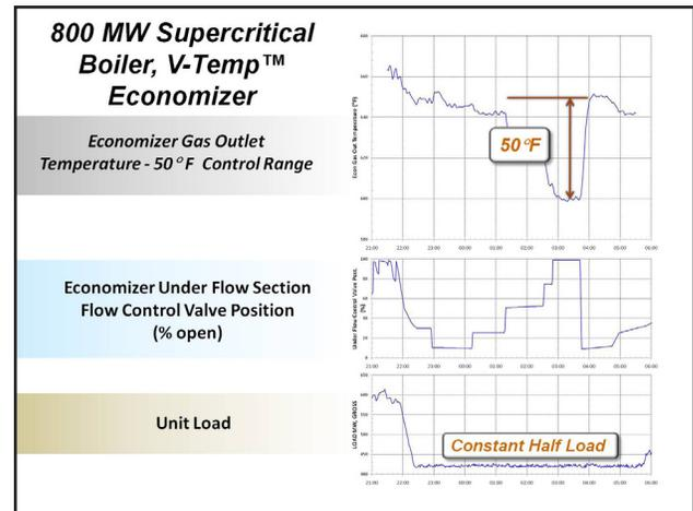
Fig. 11 V-Temp economizer test control range.
