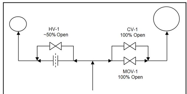
**Fig. 8** Valve positions – start-up to minimum load required for SCR operation.
