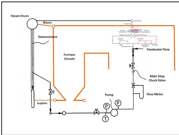
Fig. 13 Furnace/downcomer recirculation system.
