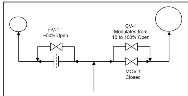
**Fig. 7** Valve positions – loads below the SCR MAIT to minimum load required for SCR operation.
